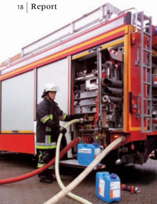
FIRESORB® in use. The product is mixed with water using a water-driven dosing pump.
