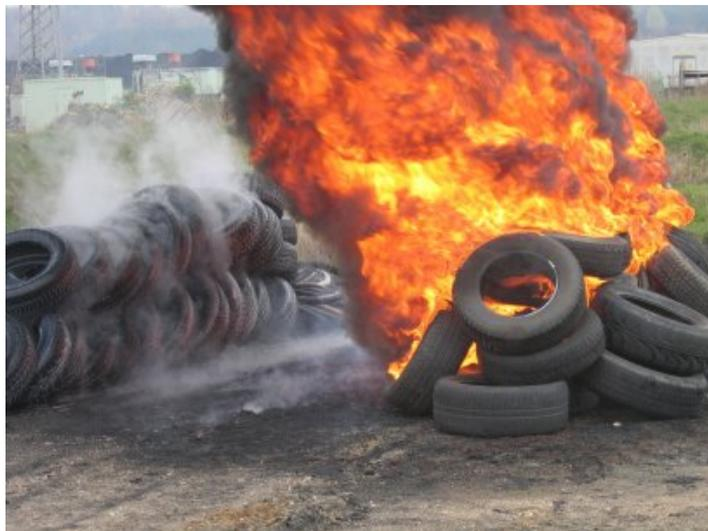
The flames did not spread to the tyre pile which was covered with FIRESORB® gel
