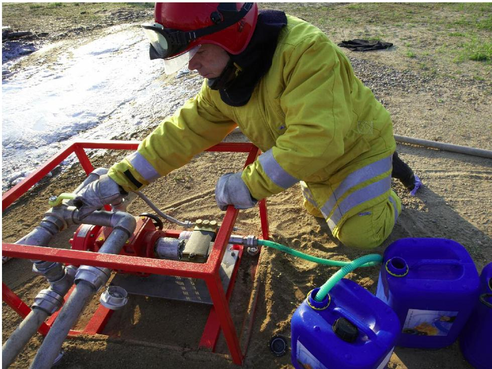
**Easy to handle – the Firesorb® concentrate can be easily mixed into fire-fighting water by stirring or pumping. The finished gel then comes out the end of the pipes or hoses ready for use. The special dosing equipment FIRE-DOS enables the concentrate to be added to the stream in a continuously variable flow of between 0.5 and 3 percent by volume. These tiny amounts are fully sufficient to generate an enormous extinguishing and protective effect.**
